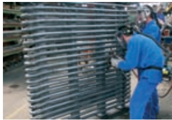
production of cooling spiral and heating coil
